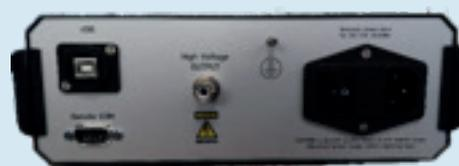
AC input : IEC 320 type AC connector fuse (L 500mA)
